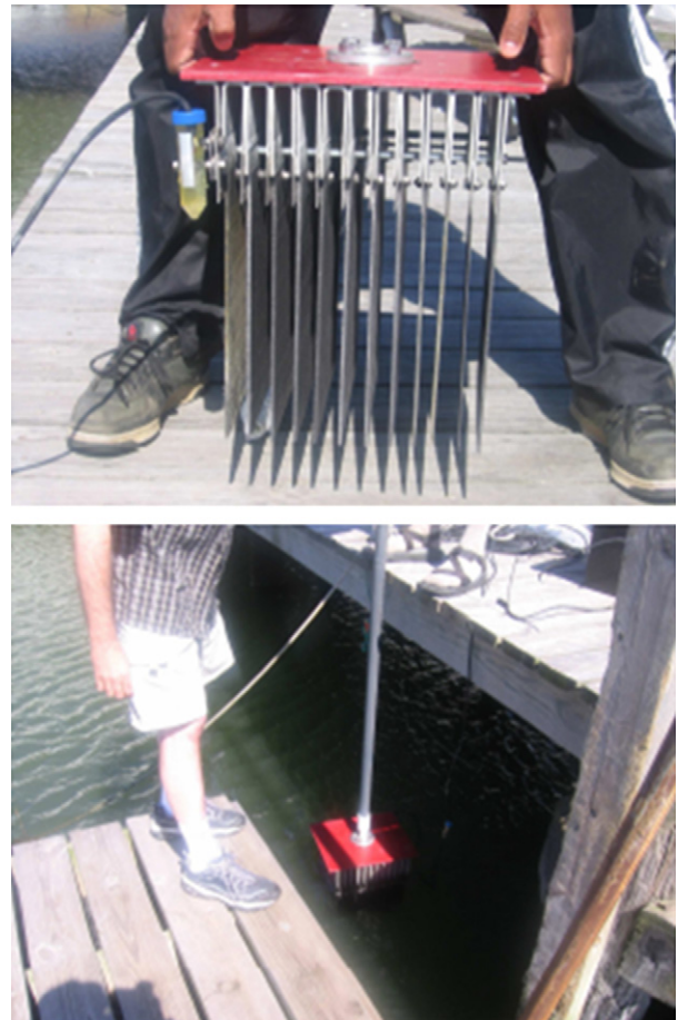
Fig. 3. Top: 12-baldd graphite anode array of second generation BMFC used to power buoy on pier at Rutgers University Marine Field Station, Tuckerton, NJ. Bottom: testing of anode embedment by impalement.
