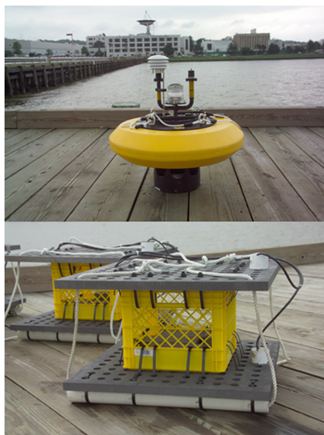
Fig. 1. Top : meteorological data buoy used in demonstration on the pier of the Naval Research Laboratory in Washington, DC, being prior to deployment (mooring and RF transmitter antenna not yet configured). Bottom : one of the first generation BMFC subunits on pier prior to deployment. Seven subunits were electrically connected in parallel to provide sufficient power to operate buoy.
